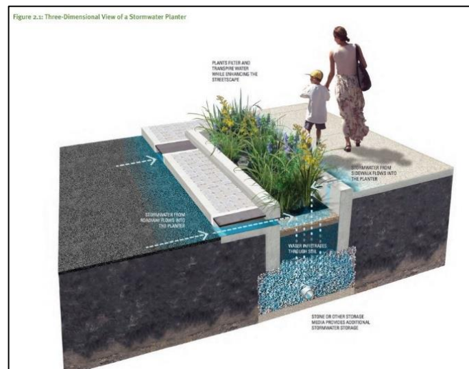
Figure 18: Street-side stormwater planter diagram
