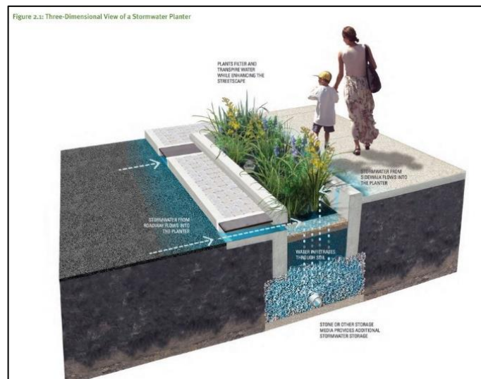
Figure 18: Street-side stormwater planter diagram Image credit: Philly Water
