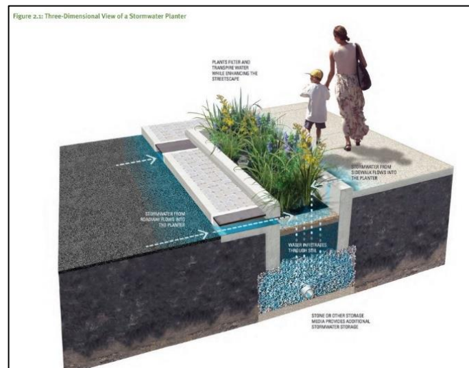
Figure 18: Street-side stormwater planter diagram
