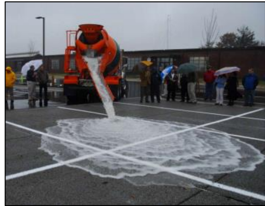
Figure 10: Rapid Infiltration of water through pervious pavement
