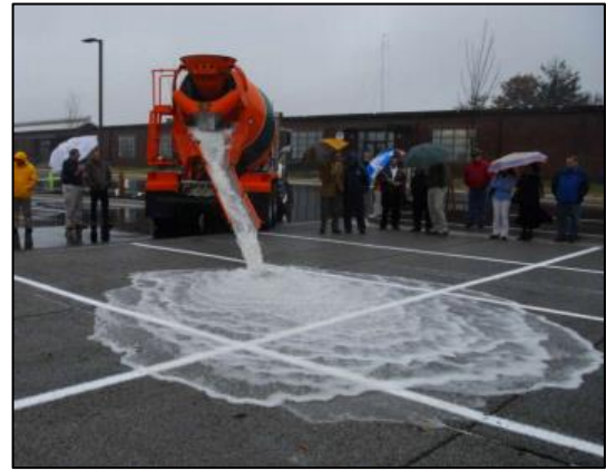
Figure 10: Rapid Infiltration of water through pervious pavement
