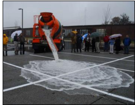
Figure 10: Rapid Infiltration of water through pervious pavement
