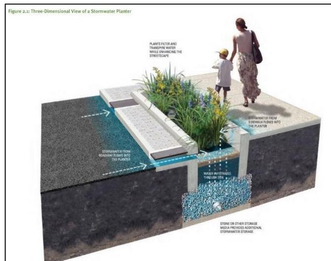
Figure 18: Street-side stormwater planter diagram
