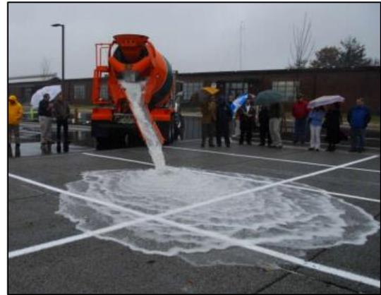
Figure 10: Rapid Infiltration of water through pervious pavement
